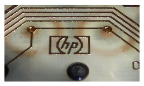
From my personal experience I know that the best remedy for electric contact problems is not just to clean contacts with solvents such as pure alcohol or lighter fuel, but rather to apply quality lubricant to contacting surfaces. So I took off the HP-41CV CPU board, and removed plastic cover sheet. Then I applied small drops of my long-time favorite high adhesive Teflon Lubricant from Radio Shack through the corresponding holes on the PC board as discussed above.
