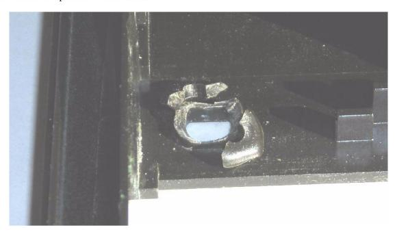
Possible explanation to this defect is the card reader. If this one is kept plugged in, and the computer is carried around and subjected to mechanical loads, this could easily lead to broken plastic. The solution to this problem was obvious: First, carefully hold together in place the loose pieces of plastic. Second, apply a drop of cyanoacrilic glue to fix broken plastic parts.
