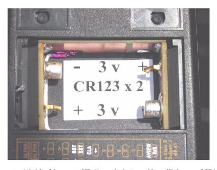
As one can see, even the potential risk of damage to HP-41 terminals (caused by unlikely case of CR123 cells' leakage) is completely eliminated with such design.
