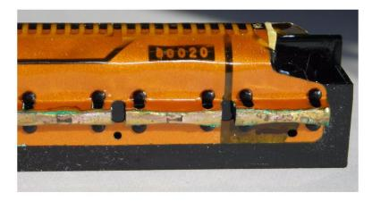
Unfortunately, battery contacts in HP-41 are too weak due to technological process used in the production (they are made not of solid metal, but rather look like thin gold plated copper traces on a thin flexible PC board). As a result, they cannot last long in principle.
