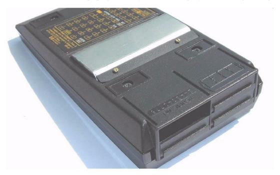
This cover is strong enough to protect HP-41 battery compartment and to absorb reasonable loads during normal use of the calculator. Insignificant excessive height of the new battery compartment lid can be compensated by using a slightly higher (by about 1 to 1.5 mm) rubber feet instead of the existing ones, if necessary (one can also keep the original feet, as I did). The steel cover is hold in place by an additional piece of plastic and two small screws, as shown in the picture.
